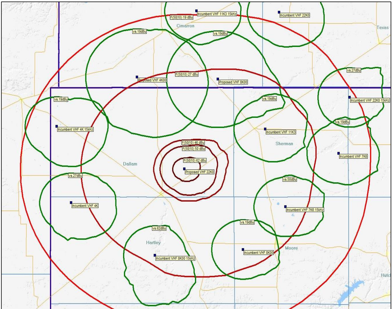
Figure 1: Results of LMCC derated contours function using ATDI Spectrum-E web application
