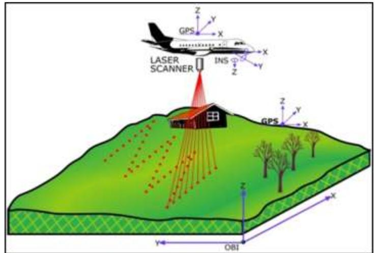
Figure 1: Airborne Lidar scanning (SOURCE: ASPRS)
