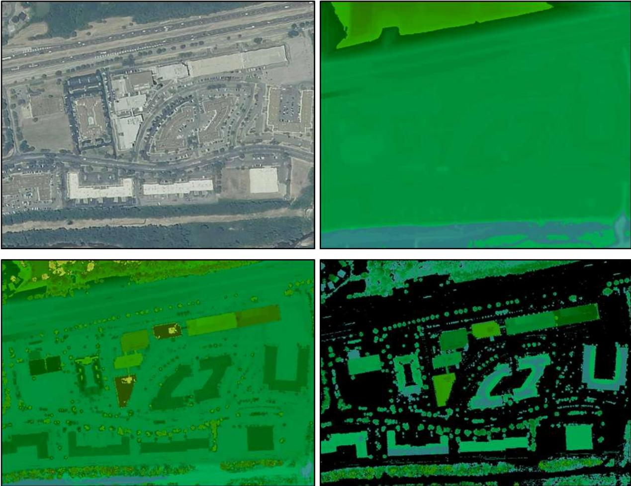
Figure 3: Aerial image (top left), bare earth (top right), first return (bottom left), and ground occupancy (bottom right)
