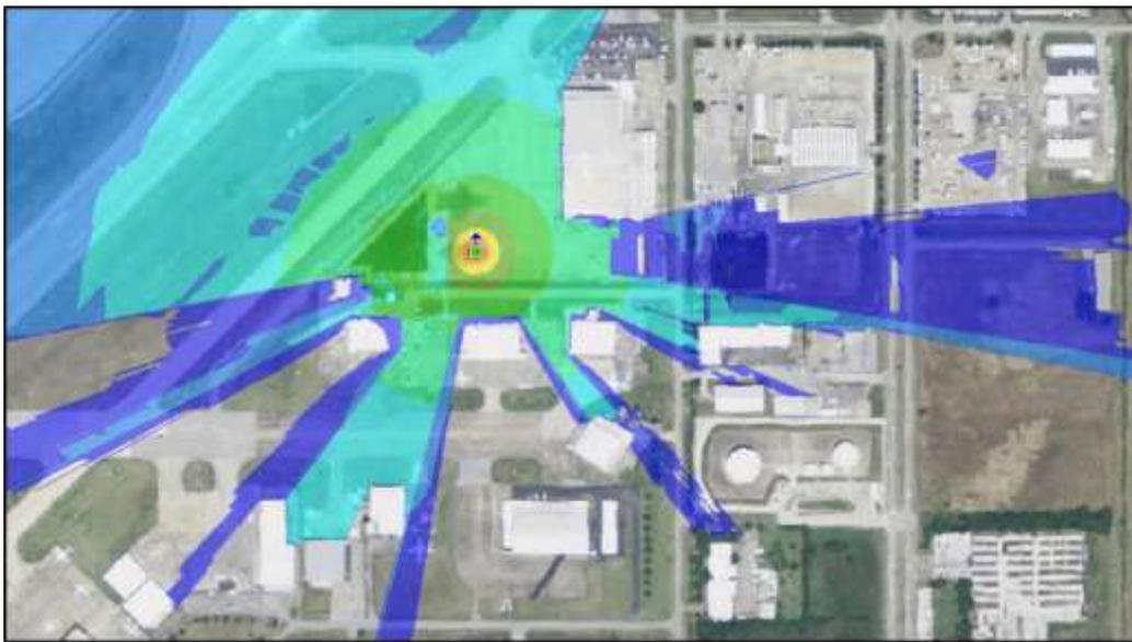
**Figure 4: Two dimensional display of RF propagation analysis results**
