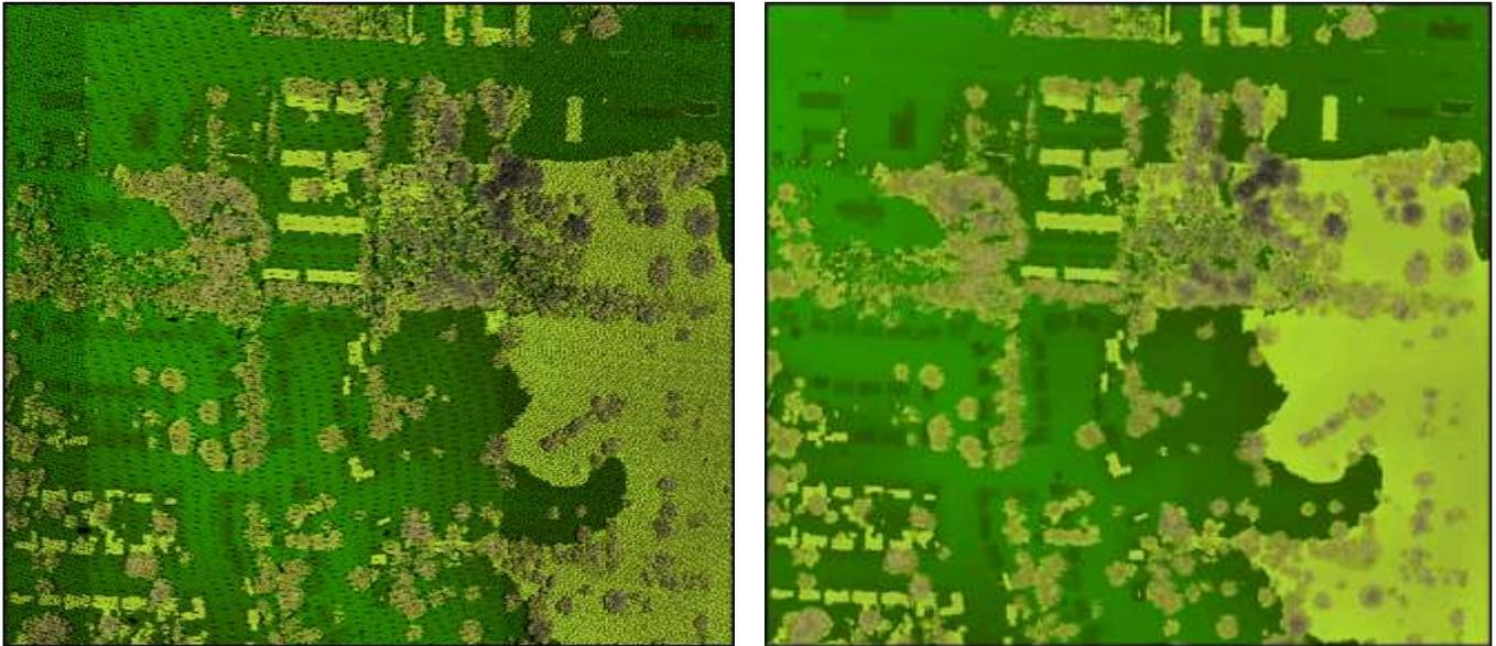
Figure 2: Discontinuous raw Lidar data (left) and continuous interpolated lidar data (right)
