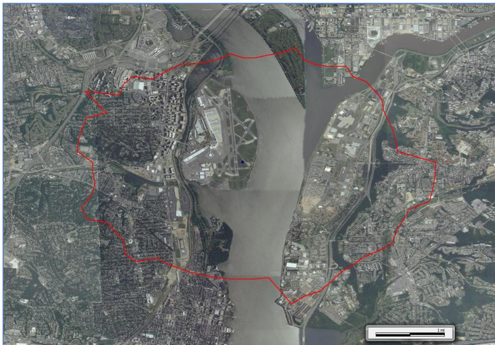
**Figure 3: Exclusion zone based on FAA 1.2 degree rule**
