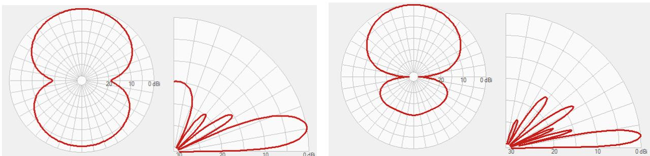
Fig 2: Same dual-band center fed half-wave dipole array, patterns at 10MHz and 5MHz
