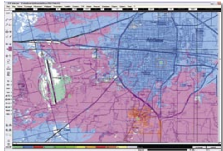
ICS telecom nG features technology oriented display : above, overlapping areas of transmitters and below, composite coverage...
