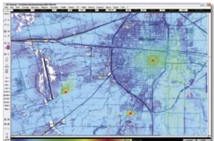
ICS telecom nG features technology oriented display : above, overlapping areas of transmitters and below, composite coverage...
