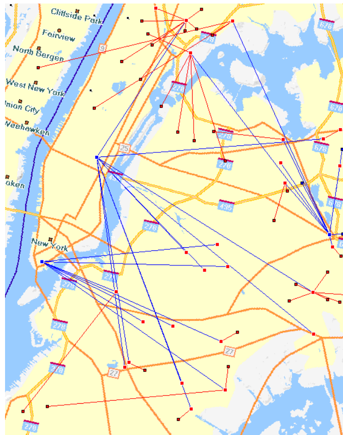
18 GHZ backhaul design with ICS telecom – Blue points represent Fiber points, red points represent existing MW towers. In this example, the tool's auto-planning features were asked to identify the best backhaul link configurations between imported Fiber locations and imported candidate MW link locations, with consideration of a single hop at most.
